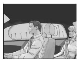
If your vehicle has one, the roof-mounted side impact airbag for the right front passenger and the person seated directly behind that passenger is in the ceiling above the side windows.
